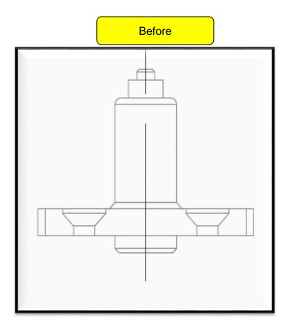
A467 Tensioner Assy. Plug Pressing Centre Locating Pin- Top Wear Out Part & Bottom Fixed Part In One Piece- Need to replace full centre locating pin after life over
