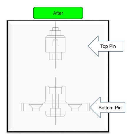
A467 Tensioner Assy. Plug Pressing Centre Locating Pin- Top Wear Out Part & Bottom Fixed Part Separate ,Need to replace full Top Pin only after life over
